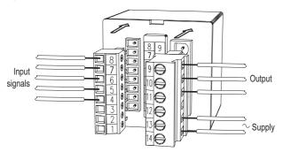
Fig.3. View of controller connection strips.
