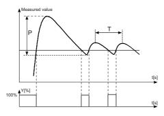
Fig.12. Selection of settings by the oscillation method.
