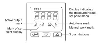
Fig.6. View of the controller frontal plate.
