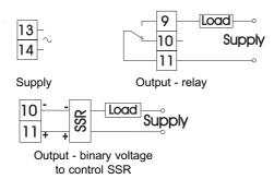
Fig.5. Connection of the supply and load circuit.
