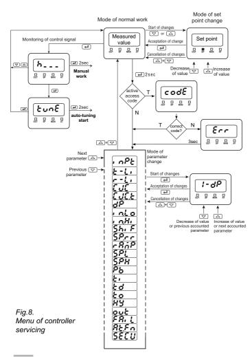
The access to parameters can be protected by a code. If the safety code is set (parameter  $5\mathcal{E}\mathcal{E}\mathcal{U}$  is higher than zero), one must give it. If the value will not be given or will be erroneous, the inscription  $\mathcal{E}_{\mathcal{C}\mathcal{C}}$  appears on displays, and the user will be only able to monitor parameter values.
